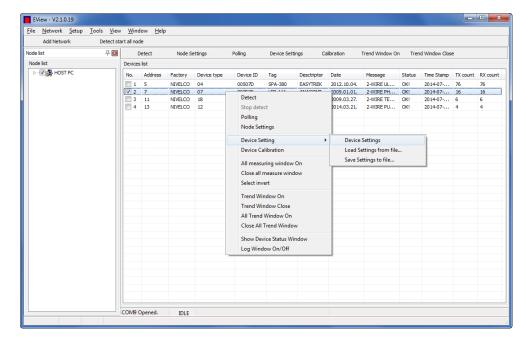
The commands of the popup menu such as Detect, Stop detect, Polling On/Off, and the Node settings has exactly the same function as the equivalent quick buttons in the menu bar.
