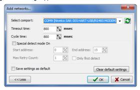
Tick the **Special detect mode On** to activate the special settings of the detection mode to be modified. The special settings are described in the following figure:
