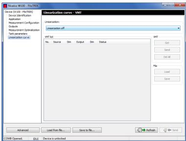
Click the **Advanced** button on the bottom left corner to reach further device settings specified for the given instrument, for example: Tag and Descriptor, Sensor info, Output and PV, Calibration, Parameters, VMT, Special, Echo map.
