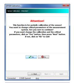
Upon that the calibration is an initial calibration or a periodic one, choose 'Yes' or 'No' to activate the Next >> button. To continue the calibration procedure click the Next >> button.
