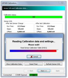
Along with opening the Sensor Calibration window the software automatically queries the calibration data and settings from the transmitter. By cancelling the parameter reading process you will exit from the Calibration window. After successfully reading the required data the device / sensor information is displayed.
