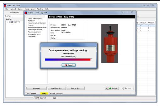
This window shows the device specific settings. The window consists of two main parts, on the left there is a navigation screen and on the right the modifiable settings are listed.
