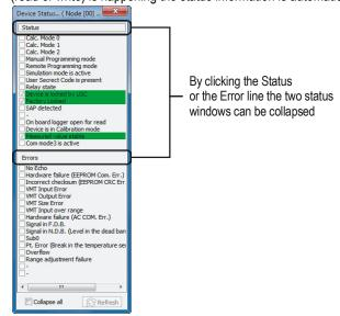
In the Status window there are device specific information displayed such as: Calculation mode, Relay operation, Factory settings, Simulation, etc..
