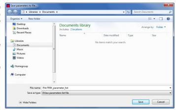
After entering the file name the clicking the 'Save' button the selected parameters will be saved to file. By clicking the 'Cancel' button or pressing the 'ESC' key we can go back to the Parameter File Editor & Viewer window without saving the parameters to file.
