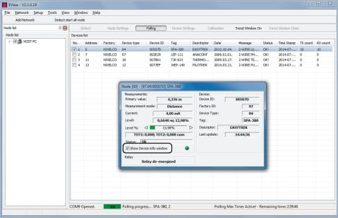
When the **Polling** button is clicked, the polling is started and the small window appears the continuous measurement data query starts. The maximum time interval of the Polling is 3 hours and the remaining time is indicated at the bottom status bar. To stop the measurement data query click again the **Polling** button. To close the Polling window untick the
