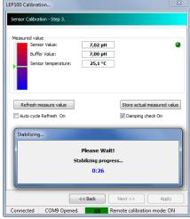
During the stabilizing progress the software queries the measurement value repeatedly and when the measurement value is stabilized (in accordance to the entered buffer value) within the given time period the software send the calibration data to the transmitter.
