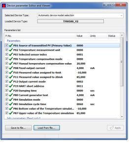
This window provides possibility to modify a parameter value in accordance to the User's and programming manual of the given transmitter. Click the 'OK' button to modify the value. When pressing the 'ESC' key or clicking the 'Cancel' button the parameter value will not be modified.
