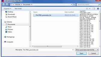
The software automatically evaluates the parameter values during the loading and checks if the values are within the acceptable range and marks the elements which has wrong value.
