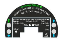
Procedure of programming: press programming keys in the proper sequence and watch state of the LEDs. See interpretation of the LEDs below ○ = LED "Off", □ = LED Blinking, □ = LED "On" lit, □ □ = LEDs blinking alternatively ⊗ = Do not care
