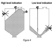
With powder level detection device should be installed at an inclination exceeding the angle of repose (or, in case of high level detection vertically), to prevent powder deposition on <sup>0</sup> vibrating rod that might substantially reduce the self-cleaning effect. Also avoid mounting the rod in a recess (see Figure 5)
