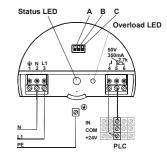
Figure 8 Electrical connection of a optocoupled sink input to a solid state output version supplied from a AC
