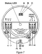
Electrical connection of relay output version
