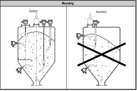
The housing can be rotated after the mounting! In case of side-mounted units, the cable glands should be downwards!
