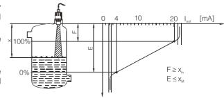
ATTENTION! When using off-site calibration, distance between the reflecting object and the unit must correspond to the required 4/20 mA values.
