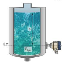
P<sub>hvdr</sub> [bar] = hydrostatic pressure
