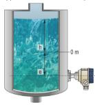
Zero point of the transmitter can be shifted up to the 50% of the range. Doing so the active measurement range will be reduced by the distance of "e"
