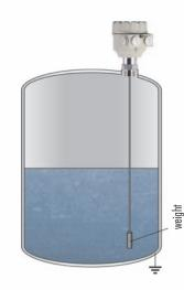
Cable probe with weight Metal tank
