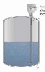
Rod probe Metal tank and non-conductive medium. The rod probe is insulated partially at the process connection.
